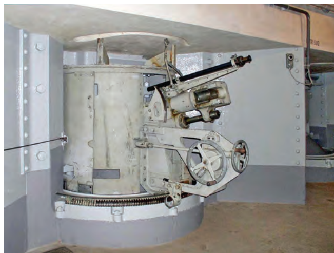
Fort du Scex: One of the 1911 double casemates for two 17.5cm L30 1903/18 guns. Photo Fortress Historique de St-Maurice
